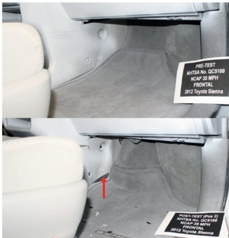
Figure 9: Pre (top) and Post(bottom) crash photographs of the right front footwell of a 2012 Toyota Sienna (NHTSA test #7615). The red arrow in the post-crash photograph illustrates the approximate location of the ACM. Based on the photographs, there was significant intrusion and deformation in the area of the ACM.
